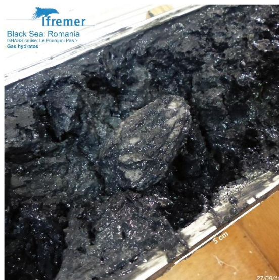
Figure 4: Close-up showing a gas hydrate nodule surrounded by severely damaged clays in core GAS-CS14.
