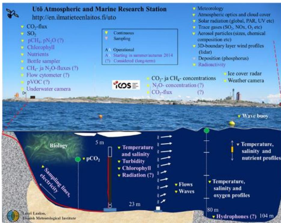
Figure 3.4: Illustration of the Utö observatory.
