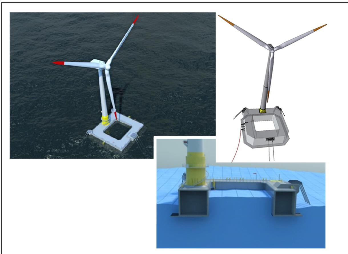
Figure 7.1: Ideol floating offshore wind turbine (credit: Ideol).
