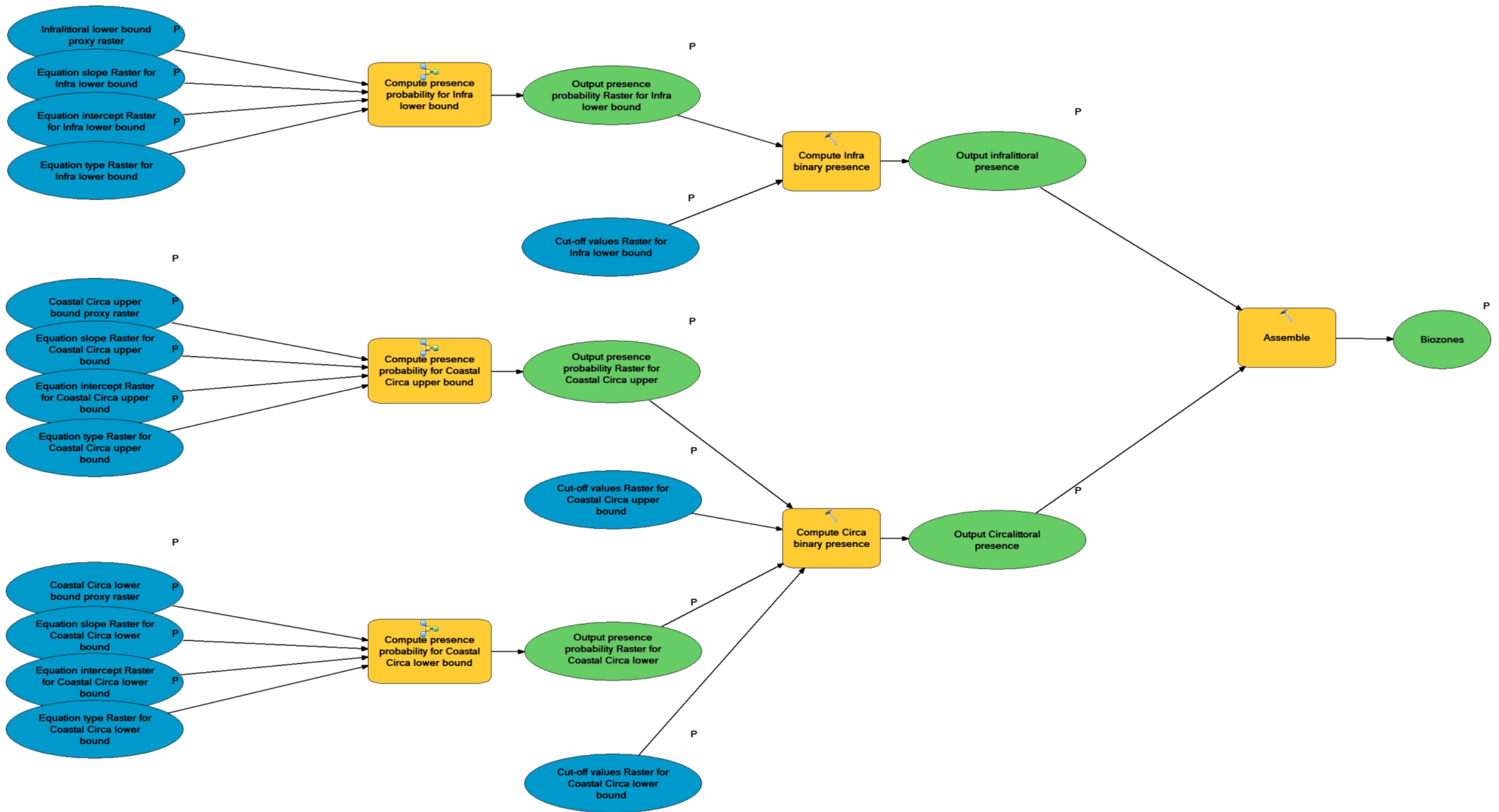
Fig. 12.4: the GIS workflow for the production of a habitat descriptor layer, namely biological zones. For simplification only 2 biological zones are considered (infralittoral and shallow circalittoral); 1: calculation of the probability layer for each habitat descriptor class boundary (infralittoral lower boundary, shallow circalittoral upper boundary, shallow circalittoral lower boundary); 2: calculation of the presence layer for each habitat descriptor class; 3: combination of all presence layers into an single categorical layer
