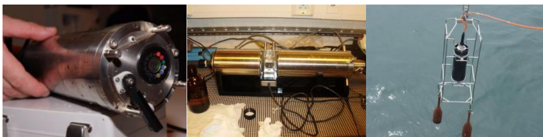
Figure. 3.2.4. Commercial spectral fluorometers: Multiexciter (left), FluoroProbe in lab measurement mode using Workstation (middle) and FluoroProbe in profiling mode (right).
