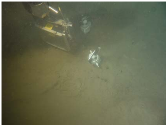
Fig. 2. Blade corer and push corers at the reference site with brown sediment covered by bioturbation.
