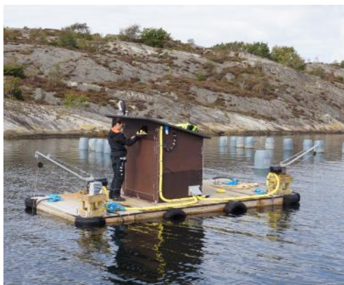
The raft at the Tångesund observatory and with winches for vertical movement of underwater microscope (Imaging Flow Cytobot) and CTD. The hut on the raft contains batteries, computers, communication equipment etc.
