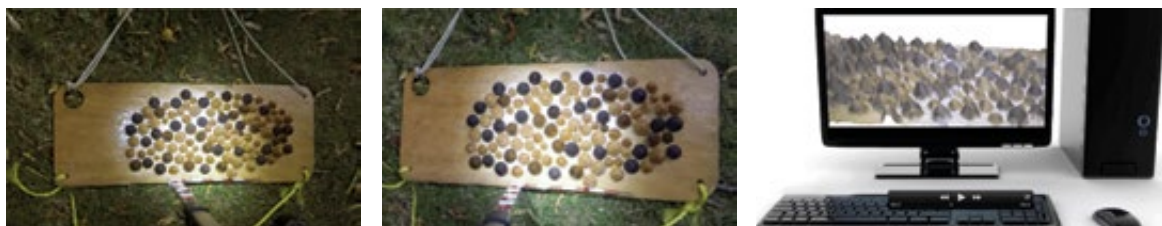
Figure 25. 3D reconstitution from 2 images in the case of a “Biocolmar®” plate with various colors and without turbidity (University of Nantes - GeM-MMS-IXEAD-Biolittoral/MaREI (Ireland)).
