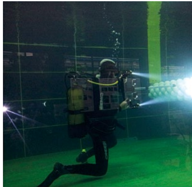
Figure 24. Tests in the Ifremer basin (Boulogne) - Financed by the company TOTAL for the validation of the protocol developed in COSELMAR for the case of mono-color roughness and absence of turbidity
