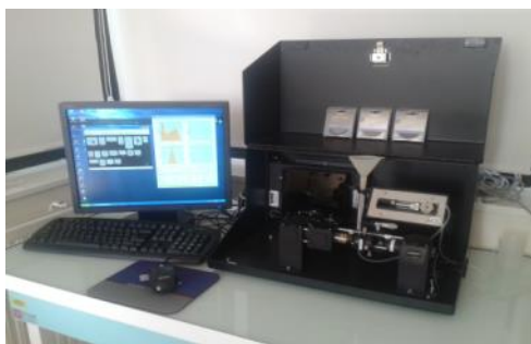
Figure 3.1.2. A benchtop version of the FlowCam. There are other versions available.
