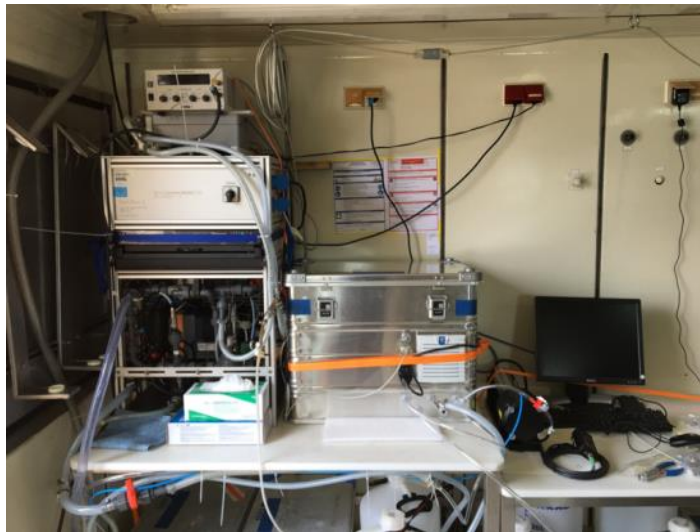
Figure 3.3.14: Sensor set-up during both cruises. From left to right: FerryBox connected to water inlet, HyAbS inside Zarges-box, Oscar G-2 inside black pressure housing
