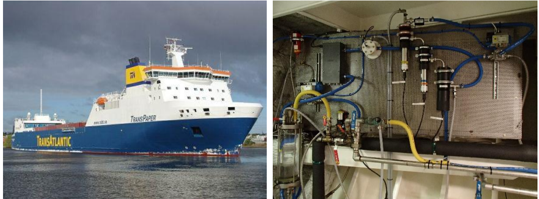
Fig. 4.1. The merchant vessel TransPaper carries cargo on the route Lübeck- Kemi-Olou- Lübeck every week. SMHI and SYKE operate a Ferrybox system on the ship. The Ferrybox system includes a pump, sensors for conductivity, temperature, oxygen, chlorophyll fluorescence, phycocyanin fluorescence and CDOM-fluorescence. Water samples for rDNA barcoding were collected from the debubbler shown in the left part of the image. Water inlet is at approximately 3 m depth.
