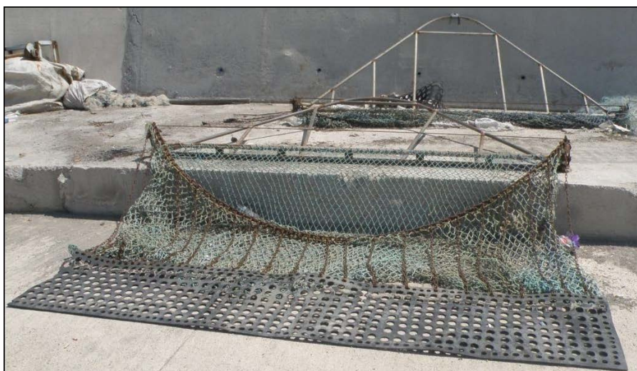
Figure 83. There is a perforated plastic/rubber palette attached to the chain on the opening of the gear, in order to mitigate the friction beneath the gear and to provide an easier slipping and also to minimize the gear deformation. Furthermore, to protect the upper panel of the gear, a covering (mantle) was added to the gear produced with a larger mesh size than of the bag and with a coarser thread material.
