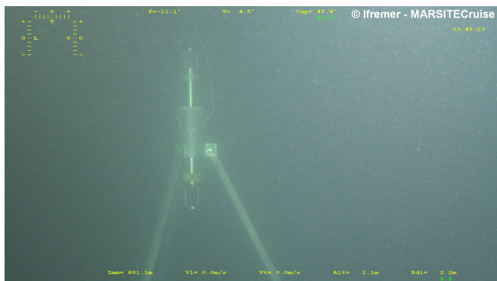
Figure I.8 Photograph of acoustic transponder installed on geodetic station G6 taken on November, 2, 2014, at 03:45 GMT with ROV Victor
