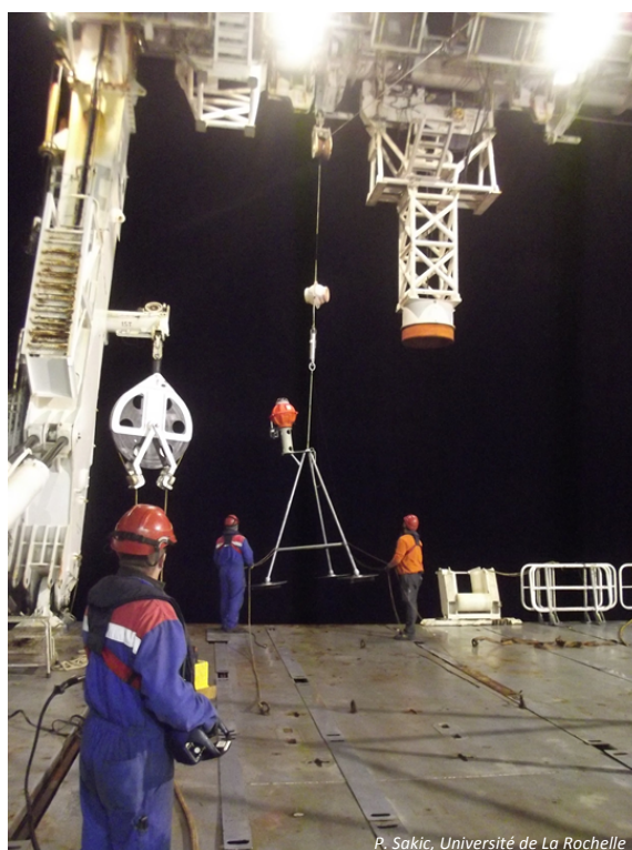
Fig I.4: Deployment of French geodetic station from R/V Pourquoi pas? during Leg 1 of Marsite Cruise.
