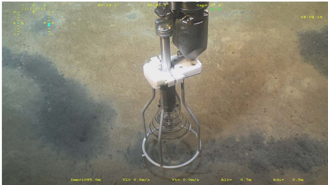
Figure 9 : Gas sampling by ROV using the PEGAZ sampler.
