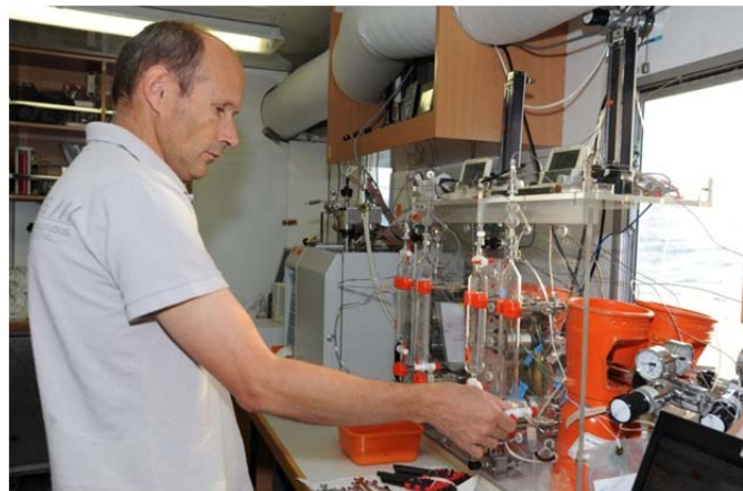
Figure 64 :: Dissolved methane concentration is measured by « purge and trap » coupled Gas Chromatography
