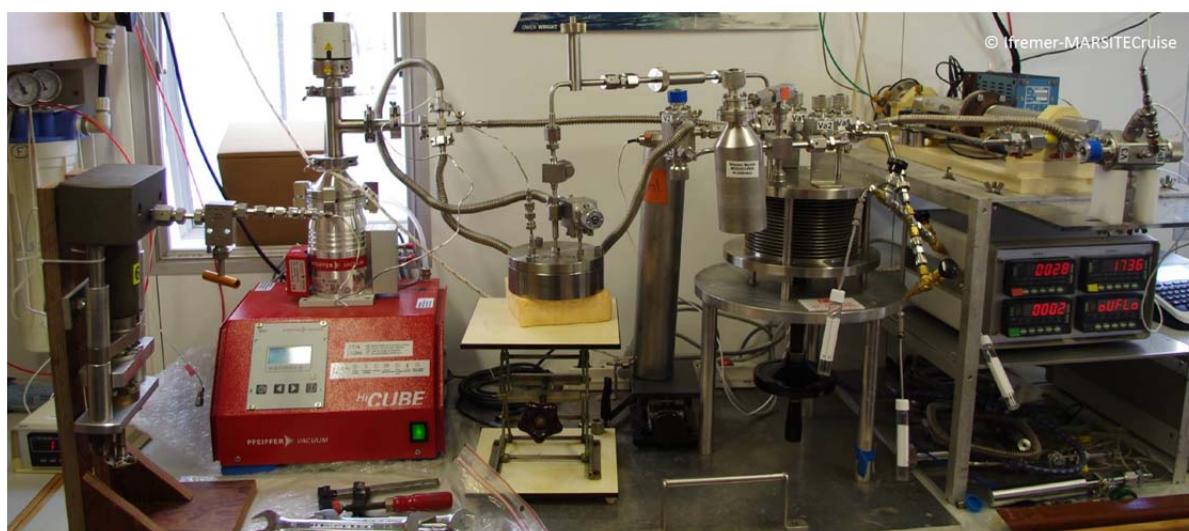
Figure 38 : Gas-extractor system used during MARSITEcruise (Courtesy of Yoan Germain)
