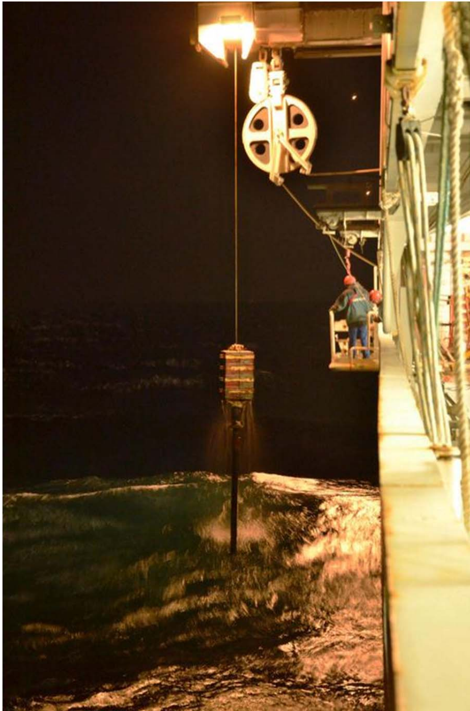
Figure 12: Recovery of a giant piston core Calypso (courtesy of Emmanuel Ponzevera)
