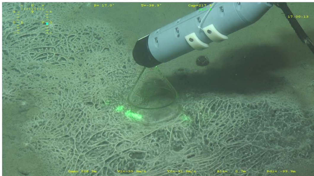
Figure 11: Chemical analysis of gas bubbles using a Raman spectrometer.
