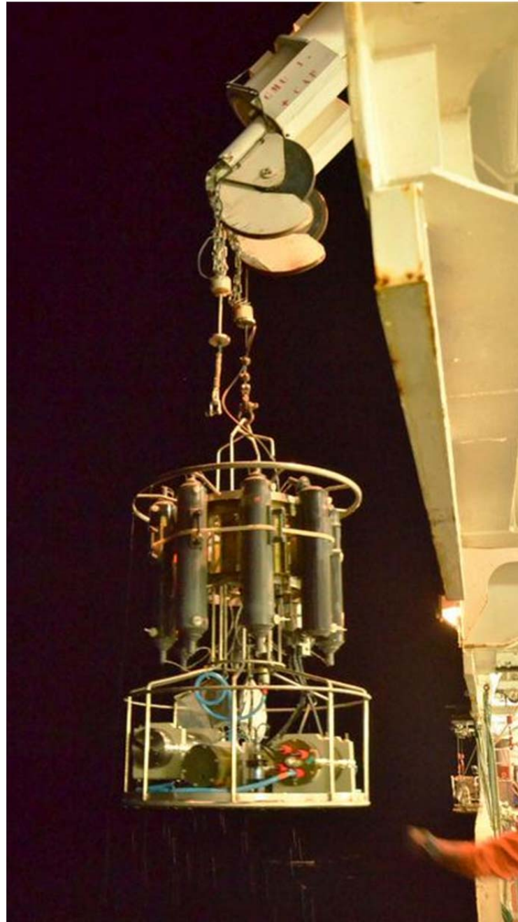
Figure 13 : CTD- Hydrocast system equipped with methane sensors (courtesy of Emmanuel Ponzevera)
