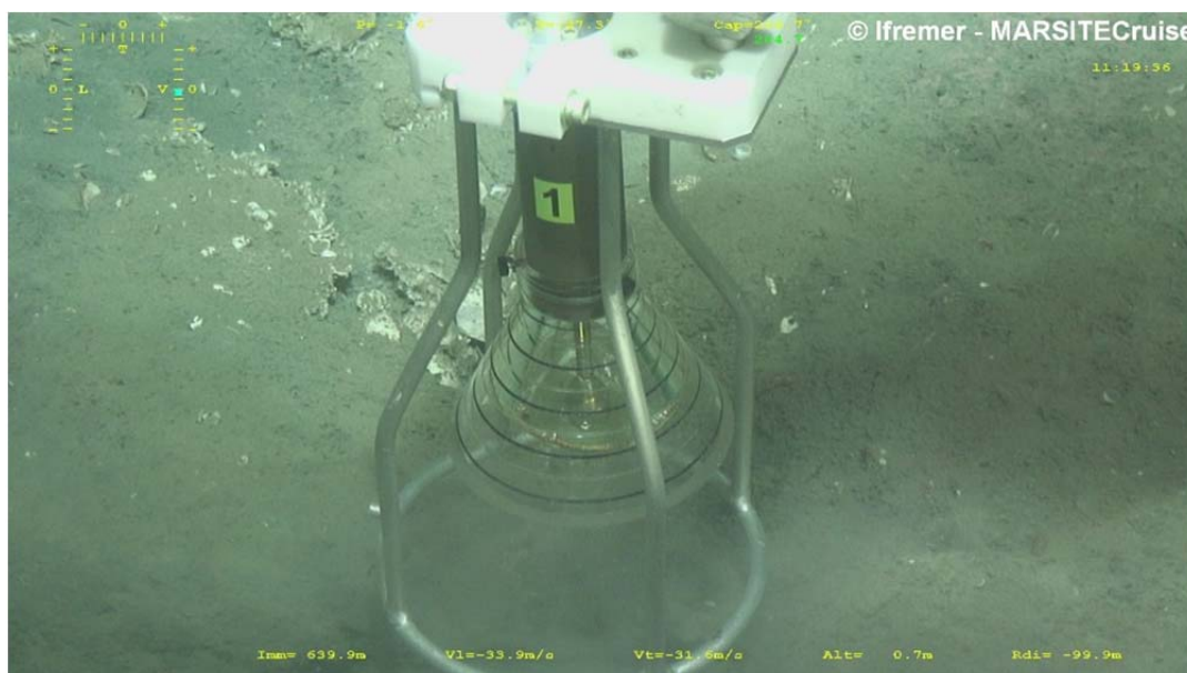
Figure 37 : Bubble sampling with Pegaz during Marsitecruise
