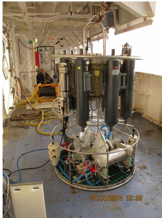
Figure 62 : CTD/ hydrocast system with the associated methane sensors
