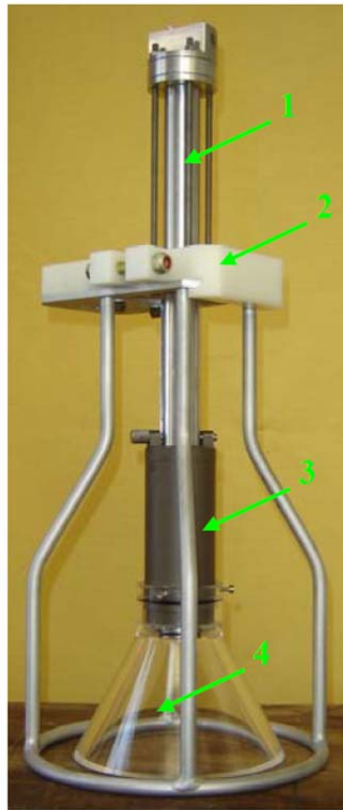
Figure 36 : PEGAZ gas-bubble sampler : 1) triggering system, 2) chassis, 3) high-pressure cell, 4) funnel
