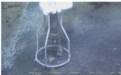
11:16 Pegaz sampling (643m) at an oil-seeping site
