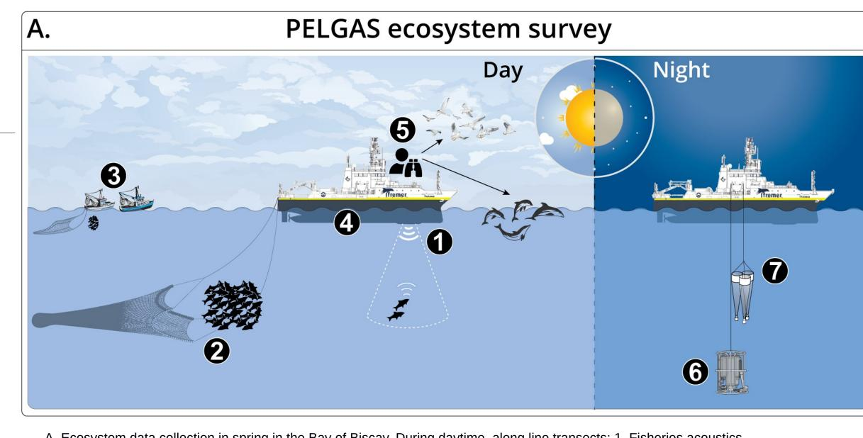
A. Ecosystem data collection in spring in the Bay of Biscay. During daytime, along line transects: 1. Fisheries acoustics, 2. R/V Thalassa midwater trawling, 3. Consort commercial pair trawlers fishing, 4. Hull-mounted thermosalinometer, 5. Megafauna sightings. During night-time, at fixed stations: 6. Sonde-based hydrobiological sampling, 7. Meso-zooplankton nets.
