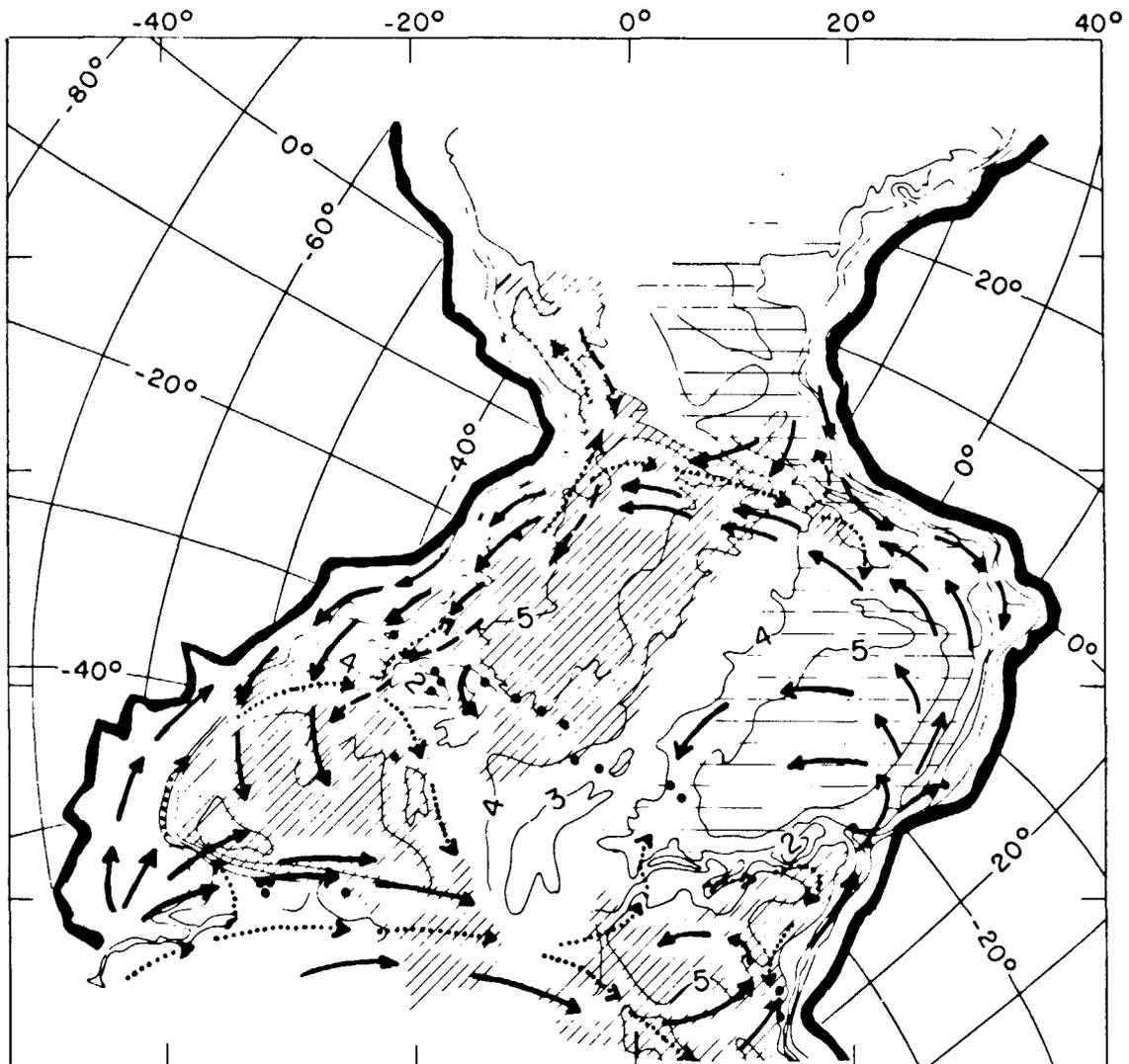
Figure 3. Bathymetric and paleocurrents map. Heavy arrows : surface currents; dashed arrows, NADC; dotted arrows, AABW. Horizontal hachures : bottom temperature greater than 1.6°C; oblique hachures, less than 1.6°C.
