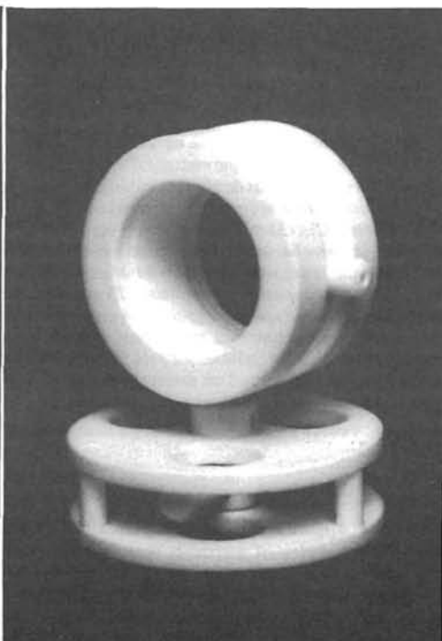
Figure 2 : Dialysis chamber on a magnetic stirrer holder.
