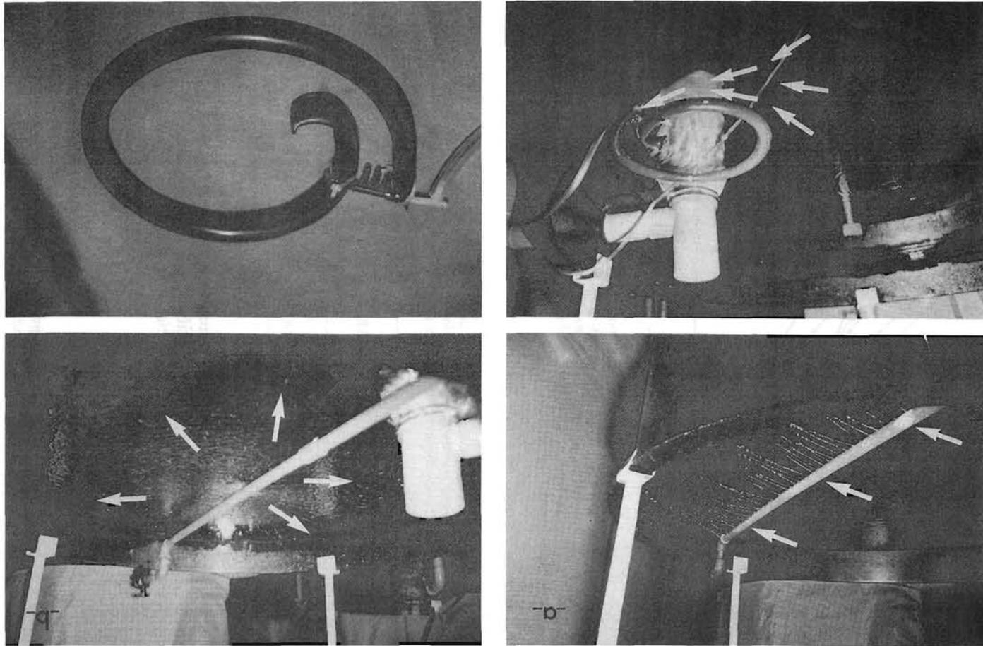
Fig. 9. — The three systems tested to remove the oily superficial layer which develops at the water surface of the rearing tanks. a : hydrojets; b : sprinkler; c and d : blower.
