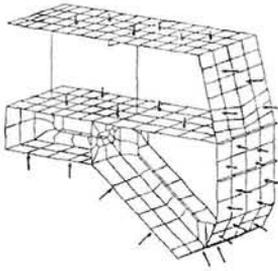
Fig. 4. Step 1 FE-model with loading
