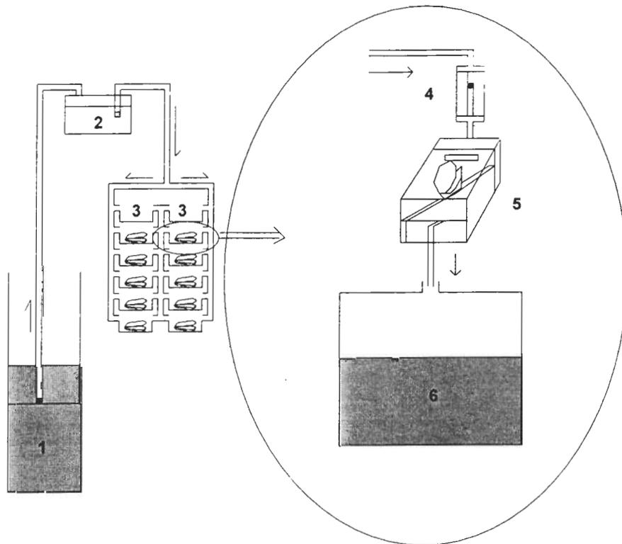
Figure 1. Experimental setup: 1, Algal (*Tetraselmis suecica*) reservoir; 2, Mixing tank; 3, set of measurement chamber; 4, flowmeter; 5, detail of a measurement chamber with oyster; 6 outflowing water collect tank.
