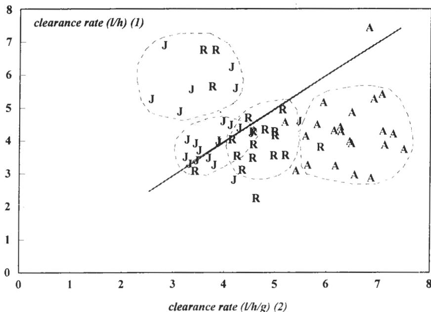
Figure 8. Oyster experimental clearance rate result (1), fitted to the clearance rate model (2):  $CLEAR = [4,825 - (0,013 \times (TEMP-18,954)^2)] \times DMW^{0,439}$  (Bougrier et al., 1995). J=ST: starvation condition; R=DS: *Skeletonema costatum*; A=DM: mixed algal diet.
