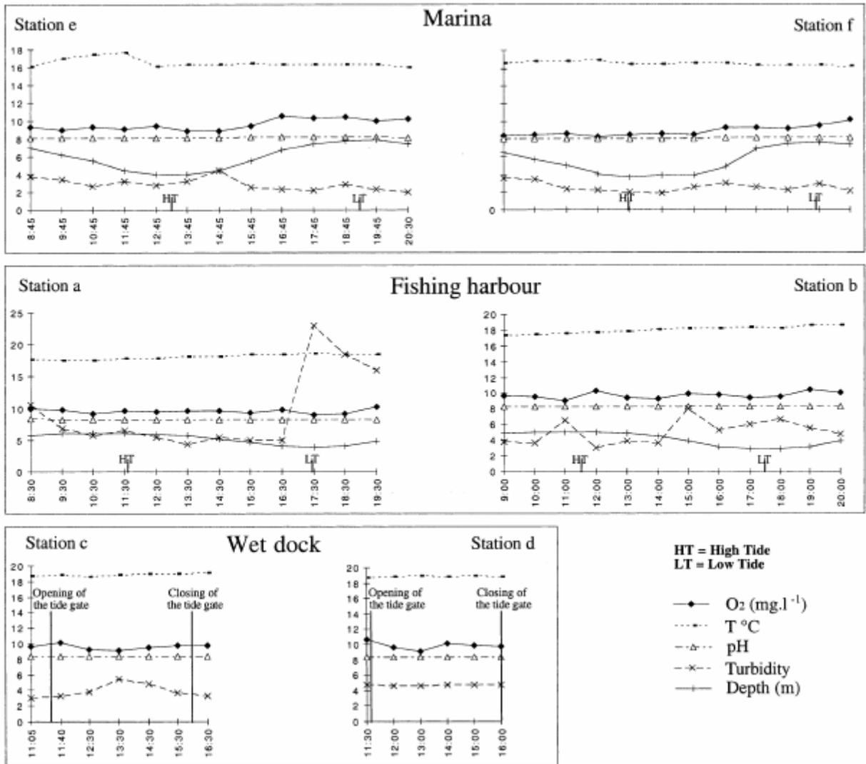
Figure 4. Variation of the hydrological parameters of the bottom water during a tide cycle.
