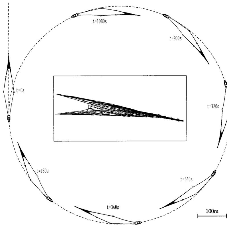
Figure 7. Trawl gear gyration
