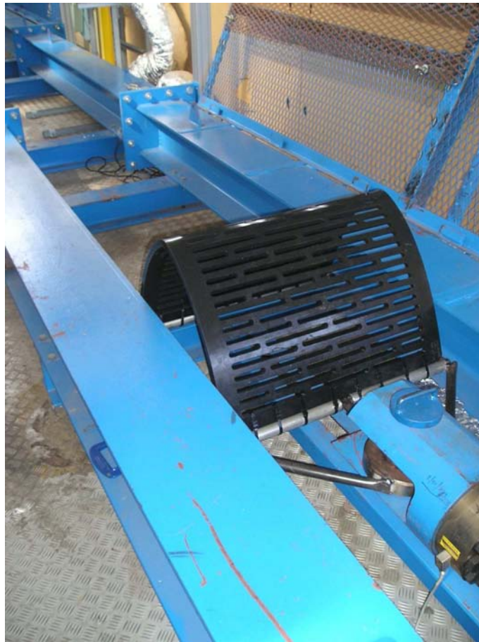
Figure 7. Grid on test frame during folding tests
