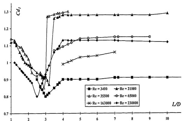
Fig. 3 Cylinders in tandem: front drag coefficient as function of spacing  $L/D$  and  $Re$
