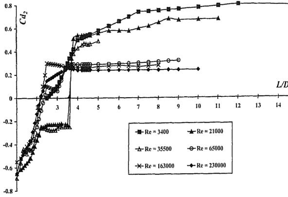
Fig. 4 Cylinders in tandem: rear drag coefficient as function of spacing  $L/D$  and  $Re$
