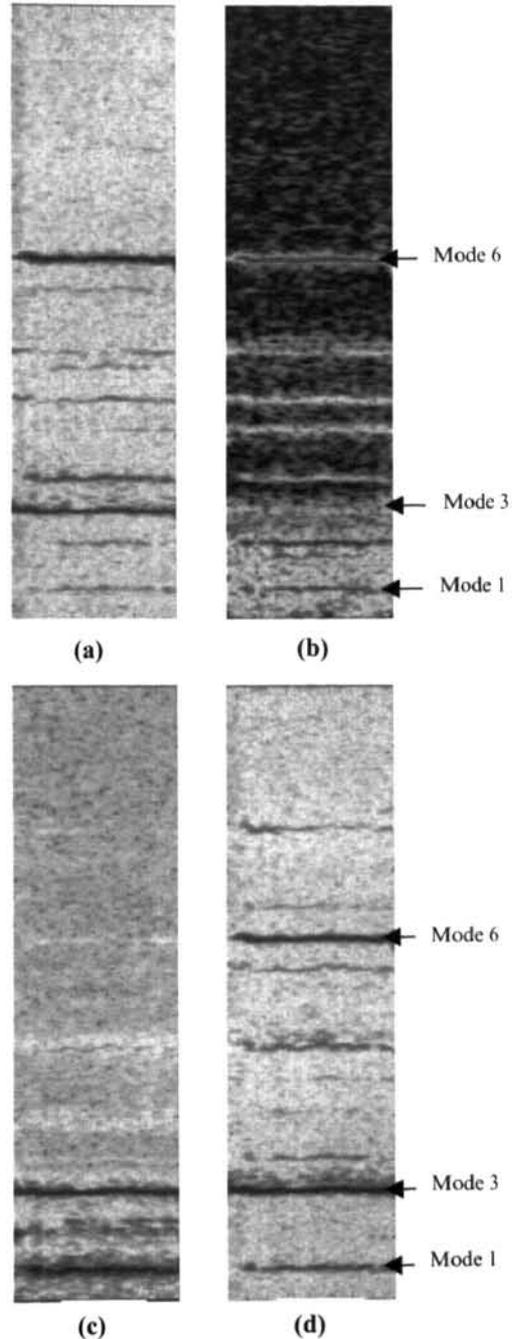
Fig. 10 Frequency versus Time for (a) inline reconstructed displacement  $X$ , (b) acceleration  $d^2X/dt^2$ , (c) cross-flow reconstructed displacement  $Y$ , (d) acceleration  $d^2Y/dt^2$  indicating fully developed statistically steady vibrations
