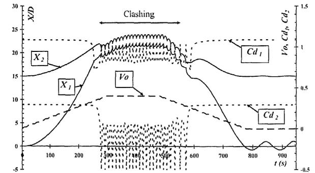
Fig. 6 Motion and drag coefficients for 2 risers in tandem in variable current  $v_0(t)$
