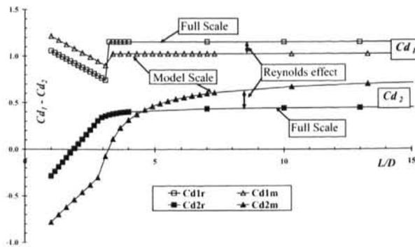
Fig. 8 Predicted spatial evolution of drag coefficient at full and model scale
