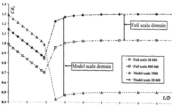
Fig. 5a Front cylinder: effect of test scaling on drag coefficient
