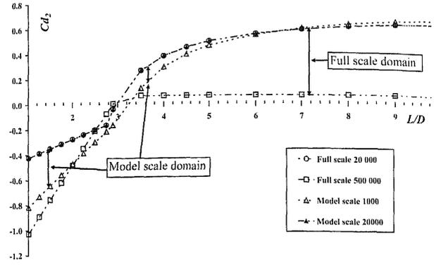
Fig. 5b Rear cylinder: effect of test scaling on drag coefficient
