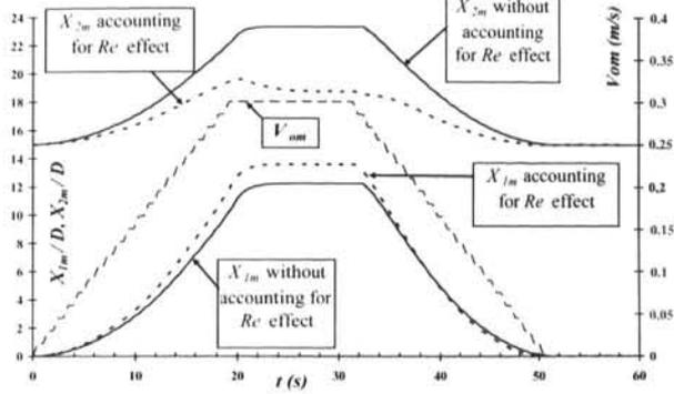
Fig. 7b Time evolution for displacement at model scale, with and without Reynolds correction
