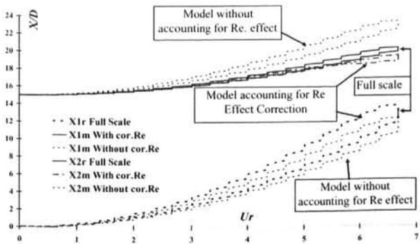
Fig. 9 Comparison of displacements at full and model scale with and without Reynolds correction
