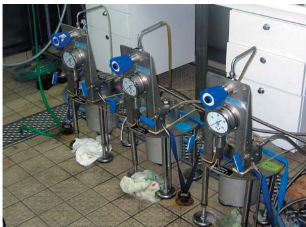
Figure 6: DESEARES (DEep-SEA RESpirometer) was used to perform in vivo experiments in simulated conditions on different hydrothermal species.
