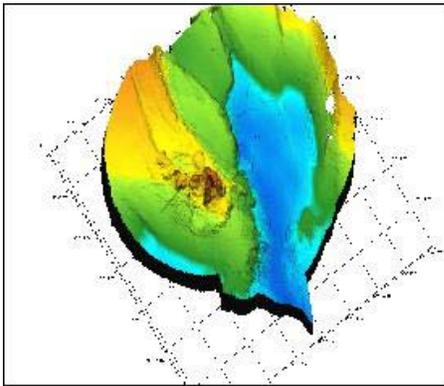
Fig. 2. A zoom on Tour Eiffel hydrothermal structure with MMR "Reson SMF 7125". Area 150m by 100m, DTM = 0.25m. The sulfide edifice is 11m high.
