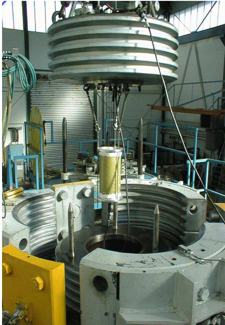
Figure 9. 2400 bar pressure vessel used for implosion tests, showing 175 mm diameter glass/epoxy cylinder before test.
