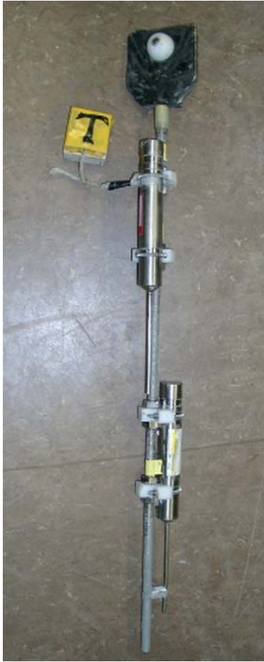
Figure 3: Mini temperature lance equipped with two MICREL temperature sensors.
