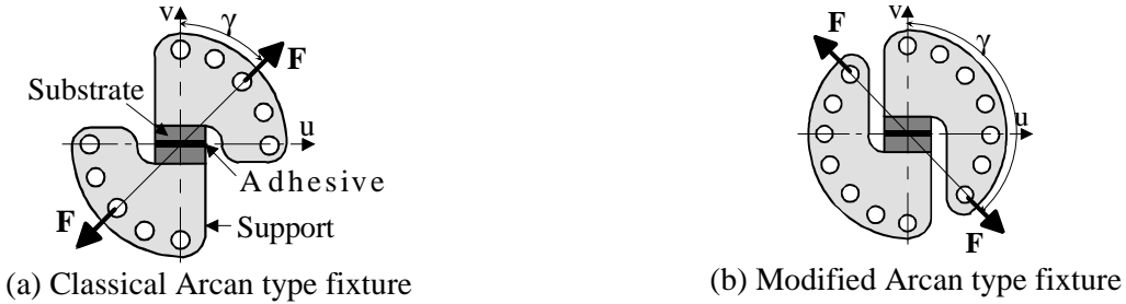
Fig. 2. Principles of Arcan type fixture.
