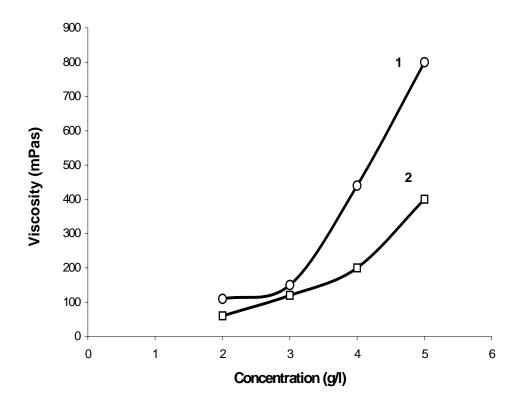
Fig. 3. Evolution of viscosity with concentration at two temperatures: (1) 30°C (2) 60°C.
