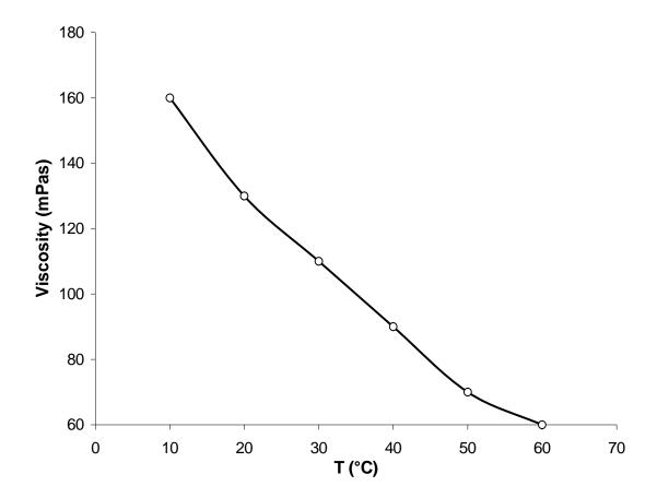
Fig. 4. Evolution of viscosity with temperature for a 2 g/l HYD 657 solution.
