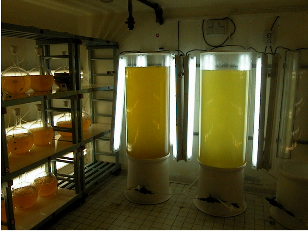
Figure 1 : Thermoregulated culture room and mass culture devices (300 L Skobalits and 10 L glass vessels)
