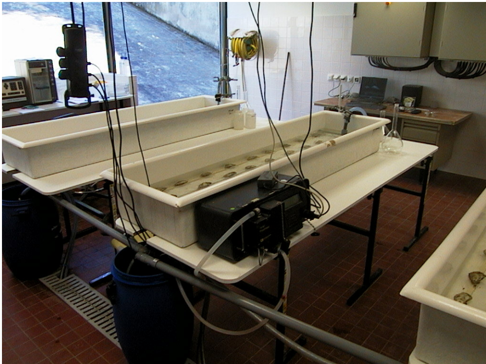
Figure 2 : General view of experimental raceways and recirculating water device used for the experiments
