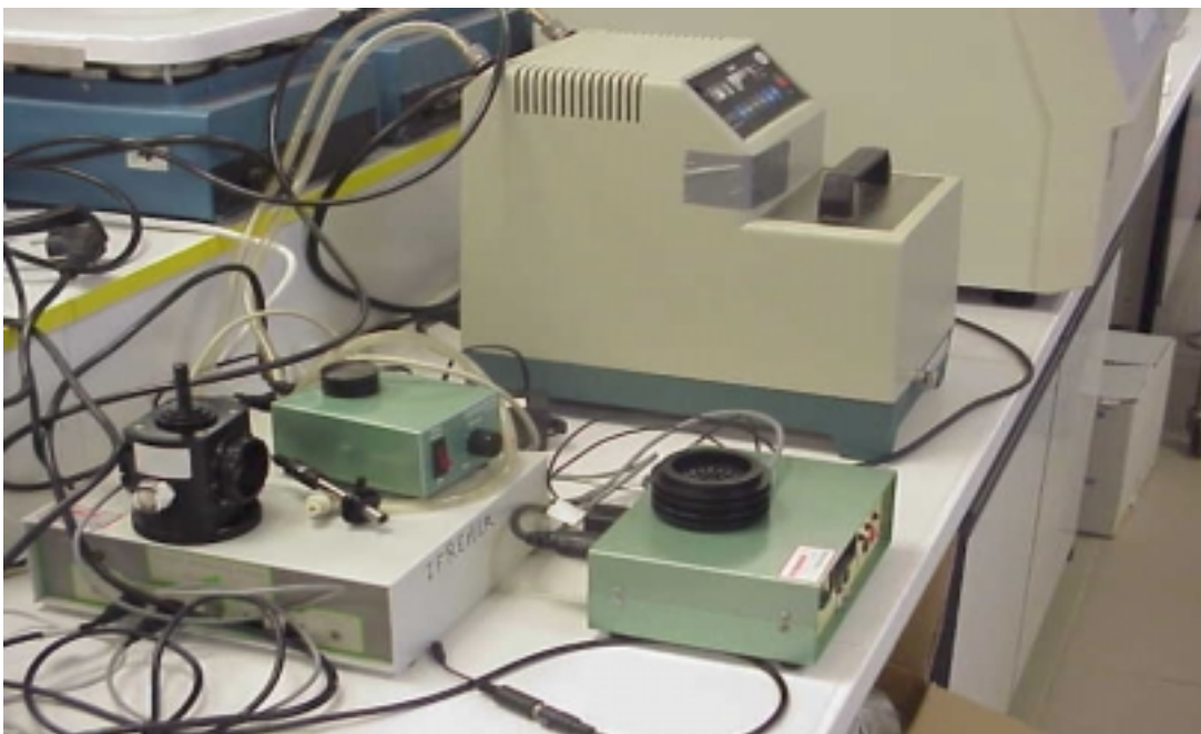
Photo III-1: L'Oxygen Monitoring System
