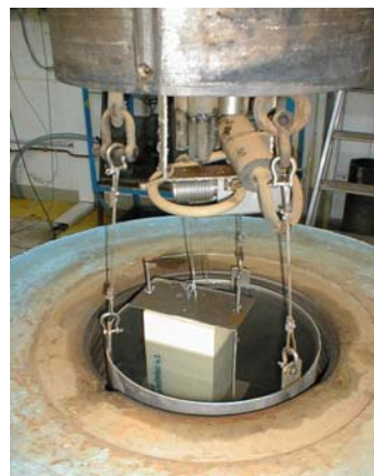
Figure 34 Test de compression hydrostatique [11]
