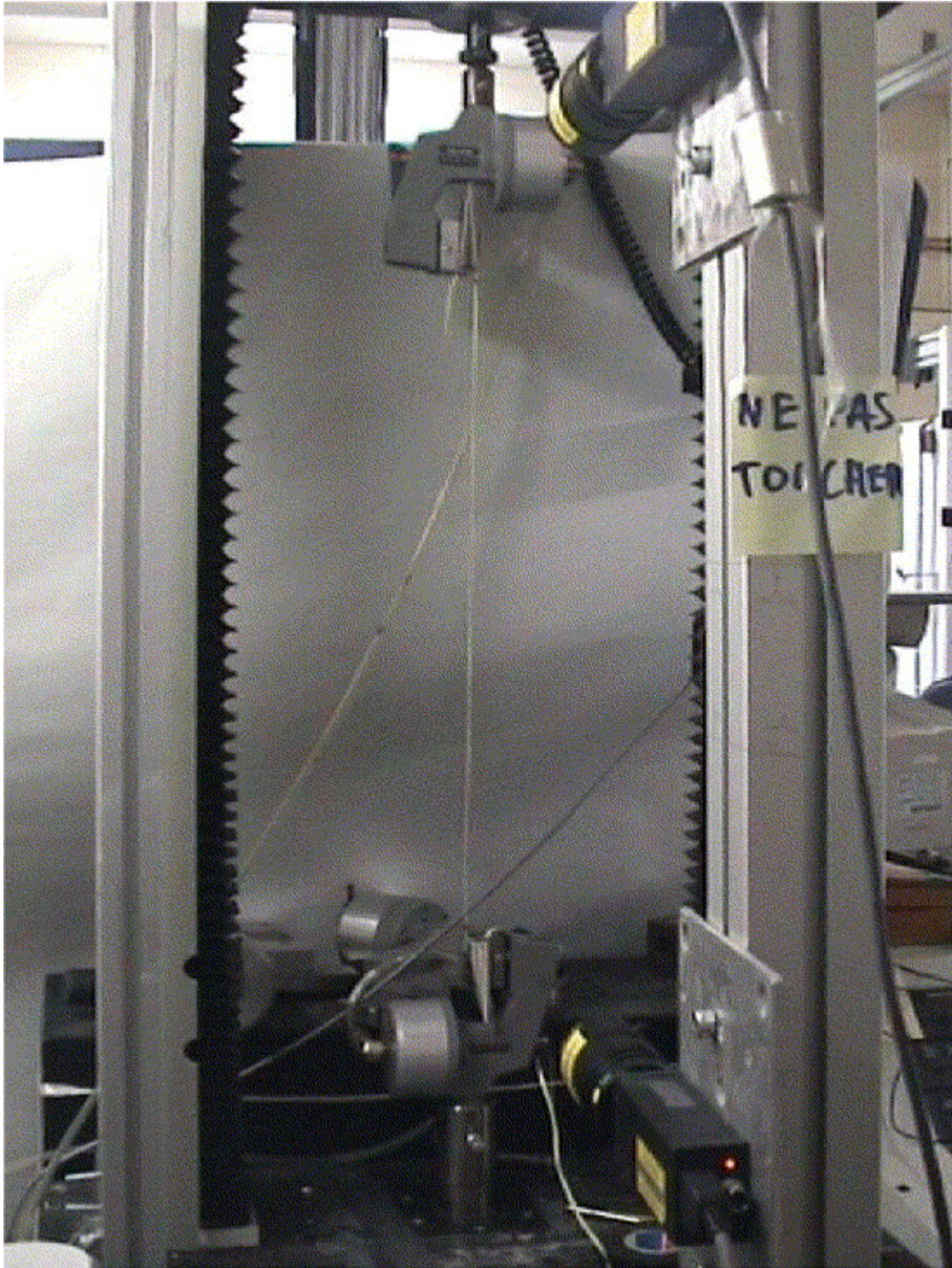
Figure 8. Testing of yarns on 10 kN test machine, two digital cameras to measure strain.
