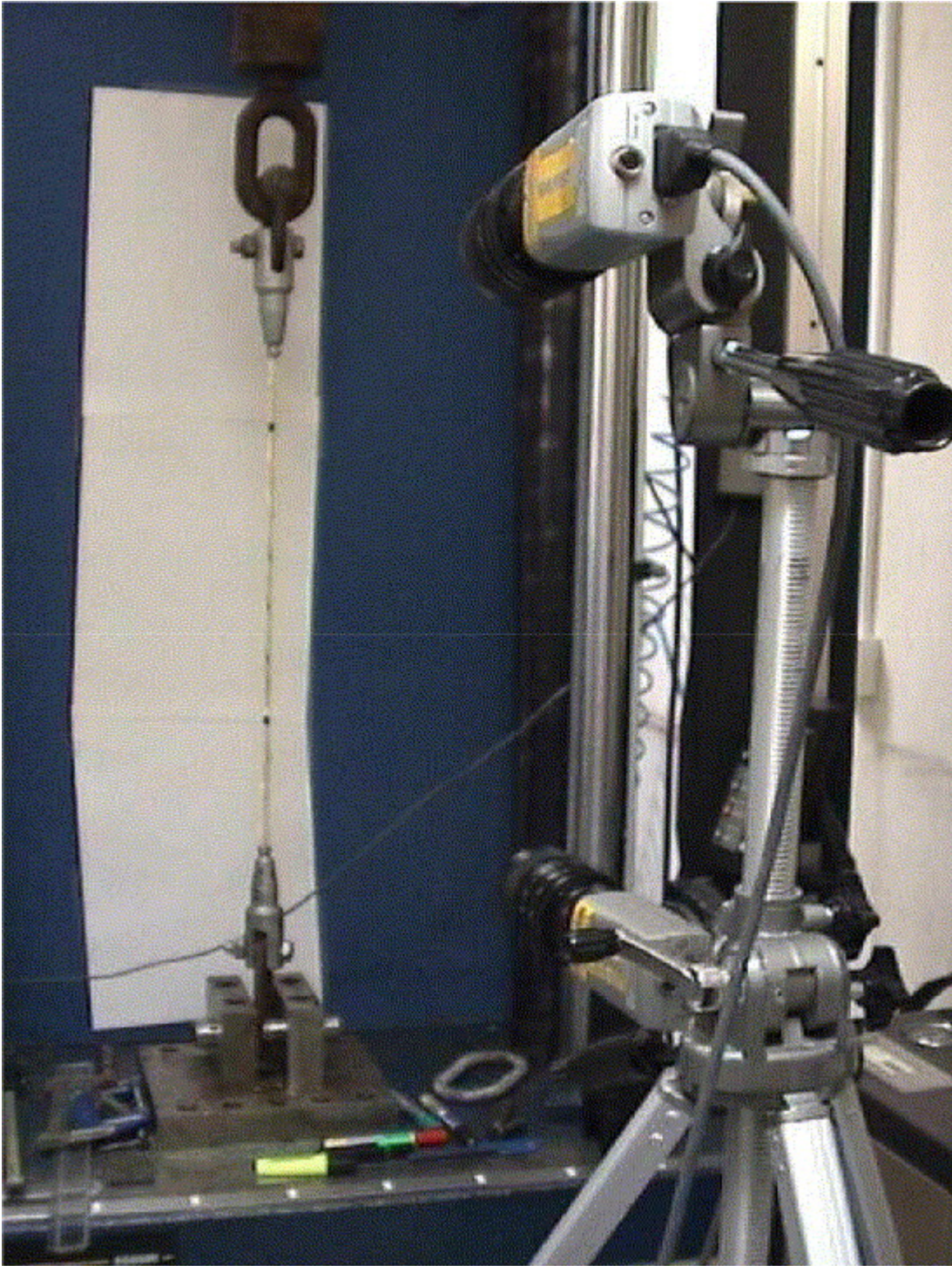
Figure 10. Test on assembled yarn sample on 200 kN test machine, showing sample and two digital cameras to measure strain.
