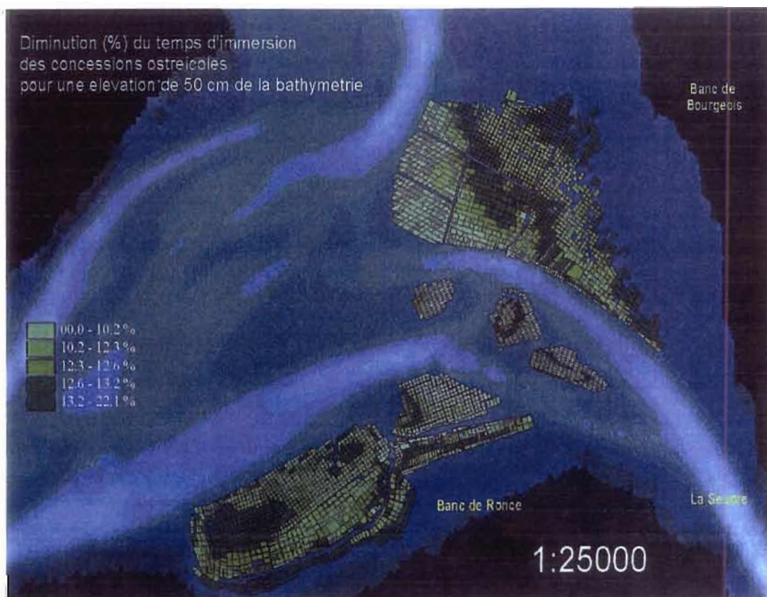
Figure N°4: Bathymetric changes (1970-1994) in the southern part of the Bay of Marennes-Oleron and simulation of oyster emersion time, and therefore filtration time decrease (%) for a 0.5m bottom rise.
