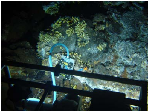
Fig. 6. The sample inlet (orange) of CHEMINI associated to two temperature probes were deployed in the mussel assemblage.
