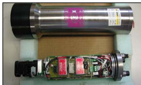
Fig. 3. Camera outside its titanium housing.
