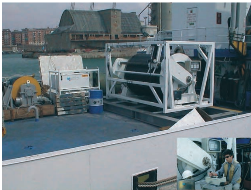
Fig. 4. The GEOSTAR handling system: power unit ( right ), cable spooled on the winch ( left ) and system console (insert) .
