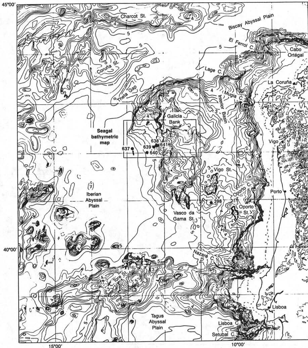
Figure 1. Bathymetric map of the Galicia Bank area (after Lallemand et al., 1985a and b). Contour spacing 200 m; for ease of identification, contours are labeled in both meters (smaller numbers) and kilometers (larger numbers). ODP sites are located within the box showing the limits of the Seagal bathymetric map.
