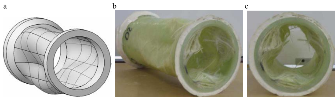
Fig. 14. Damaged thin walled specimen after implosion, showing buckling modes with mode one axial and mode 3 circumferential; (a) schematic view, (b) and (c) views of a buckled tube.
