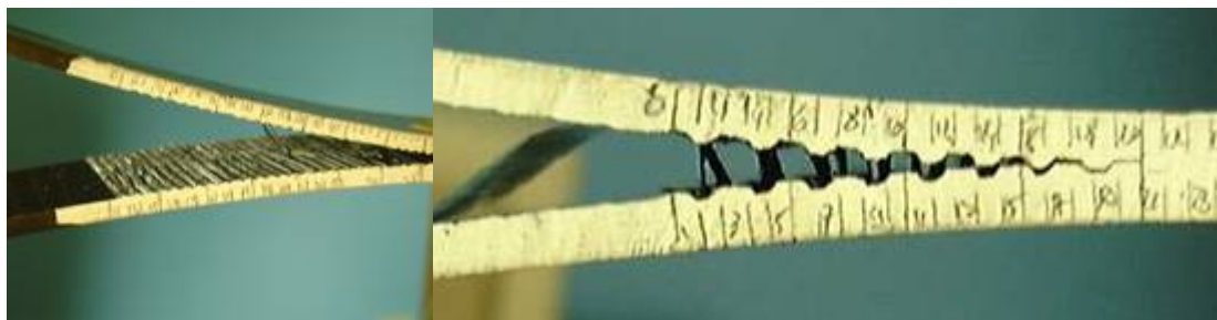
Figure 2: Typical delamination path observed in cross-ply (alternating 0^\circ/90^\circ layers) laminates, oscillating between adjacent 0^\circ plies. (Left): view onto fracture surface. (Right): edge view. If delamination paths deviate into the 0^\circ plies tests are considered invalid.
