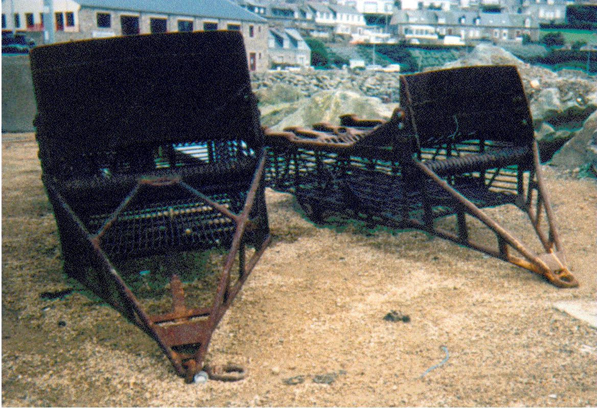
Figure 16 : Dredge with high blade of Bay of St Brieuc (from IFREMER DRV/RH).
