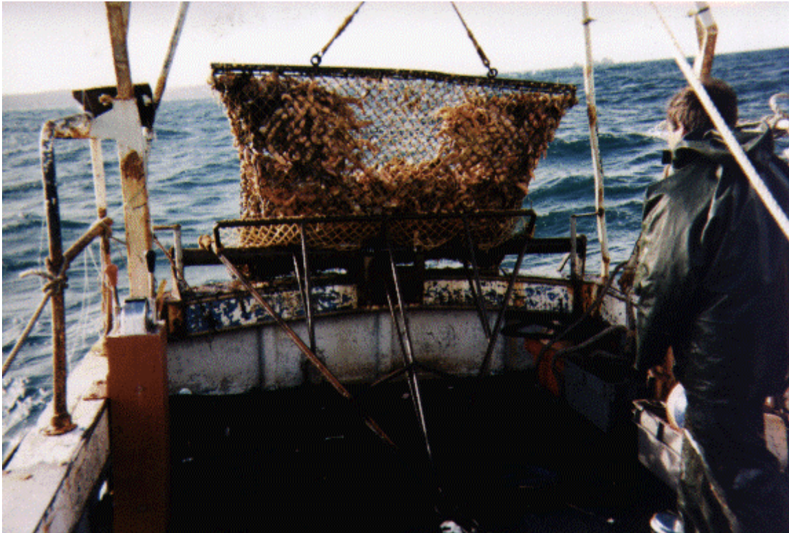
Figure 14 : Queen scallop dredge with ring bag used in the Bay of Brest and the Bay of Camaret (from IFREMER DRV/RH).
