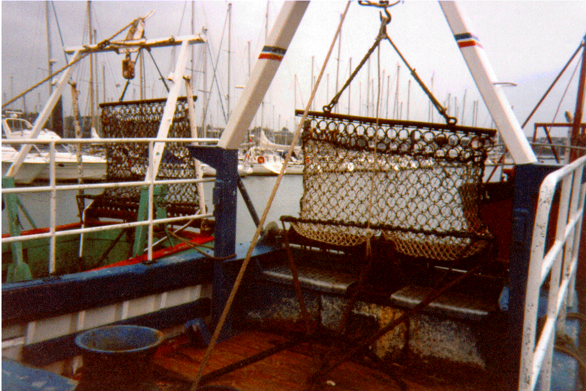
Figure 5 : King scallop dredge without diving plate in Brest harbour (from IFREMER DRV/RH).
