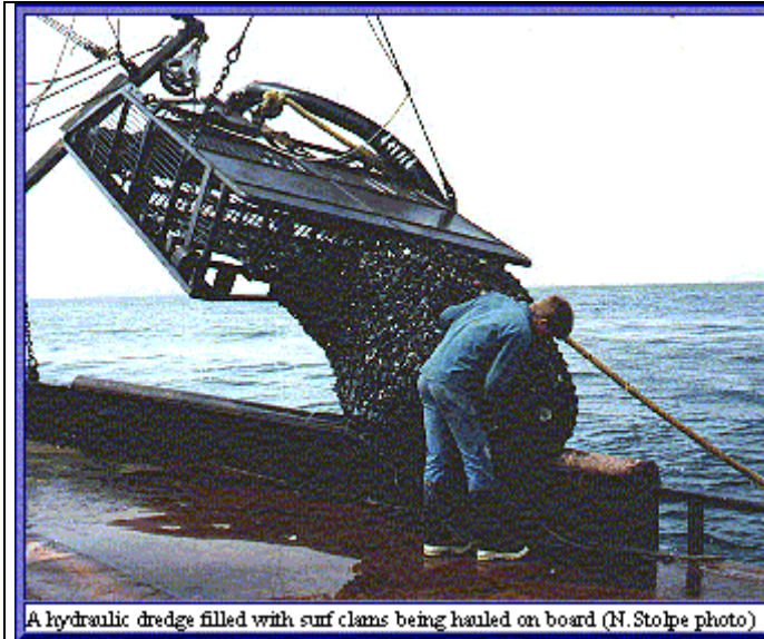
Figure 32 : Hydraulic dredge for clams of Canada and USA.
