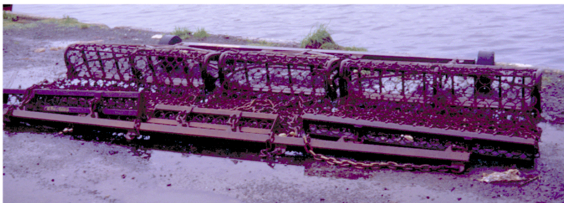
Figure 7 : King scallop dredge used in Saint-Malo Bay (from IFREMER DRV/RH).
