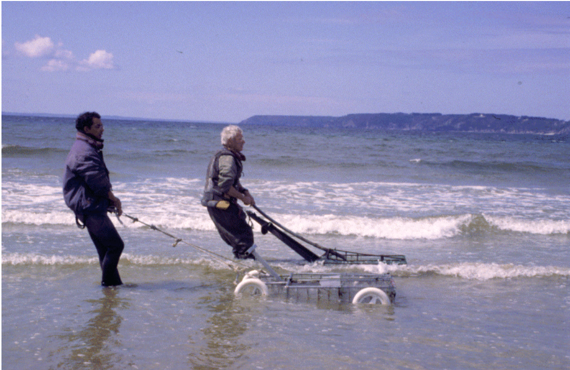
Figure 3 bis: Gear operation for manual dredge for Donax (from G. Véron IFREMER).
