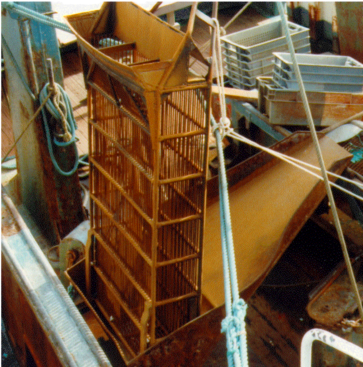
Figure 15 : Small bivalves' dredges of Granville with curved short blade (from IFREMER DRV/RH).
