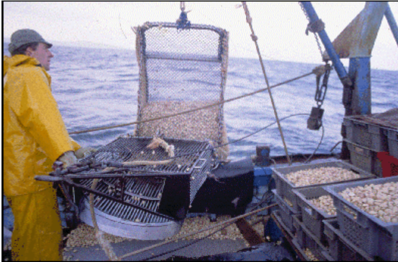
Figure 17 :Thick trough shells dredge with short blade (from IFREMER DRV/RH).
