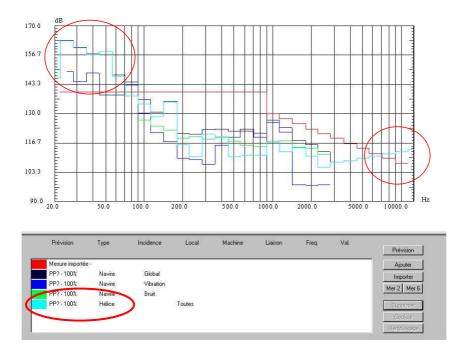
The provisional levels from the propellers are the causes of this excess. The modelling used is not yet adapted to the optimised propellers. The software is currently being improved.
