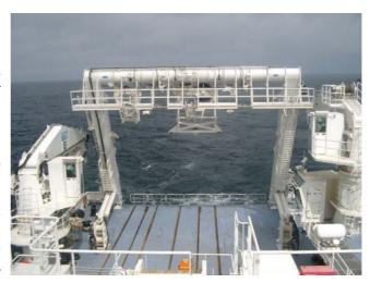
manoeuvring manned devices). It is moved by four hydraulic cylinders (two cylinders per post) to ensure stand-by redundancy should one of the cylinder fail. The submarine is lifted using a dedicated winch on the port upright of the A-frame, which is fitted with a 100mm-diameter textile hoist line.
