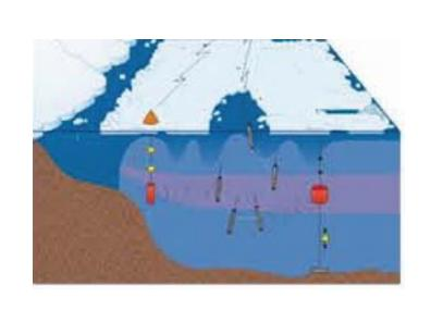
Because the Wedell Sea is ice-covered in winter the floats for this region are equiped with an Ice sensing algorithm. If the temperature in the upper 50 m is near freezing the ascent will be aborted. In this way the floats are prevented to be demaged by the ice. With Rafos floats data sampling is possible even when the sea surface is ice covered.
