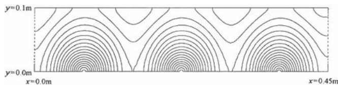
Fig. 9. Electrostatic precipitator: ion charge density distribution for (\rho_{pc})_{in} = 0 \text{ g/m}^3 and (\rho_{ion} \text{ at wires}) = 45.7 \mu\text{C/m}^3 [4].
