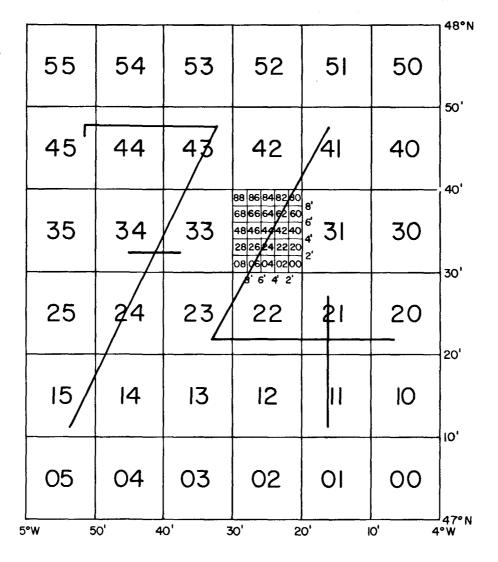
The first code figure in the proposed system signifies the latitude and longitude units. The reader will thus retain in mind the 10° units of latitude and longitude defining the work area in a general way. The data processer will incorporate these two constants in an optional program.
