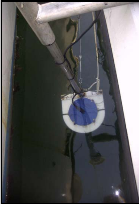
Figure II-27 : ADCP in situ
