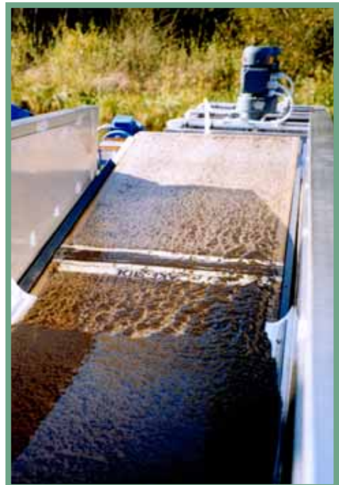
Figure 7: Belt filter in a trout farm (photo STM aquatrade)
