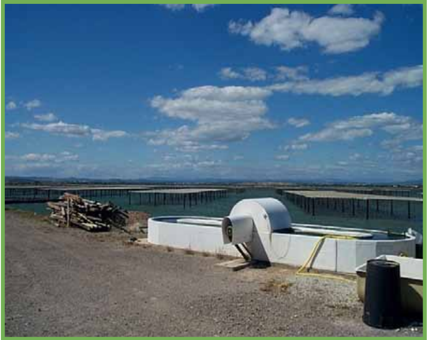
Figure 2: Pilot-scale High Rate Algal Pond (Ifremer Palavas station)
