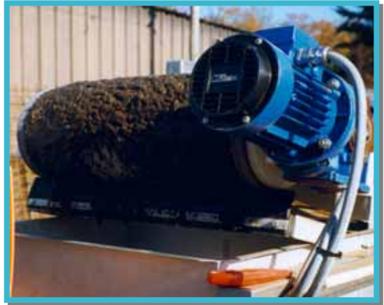
Figure 9: Thickened sludge with belt filter
