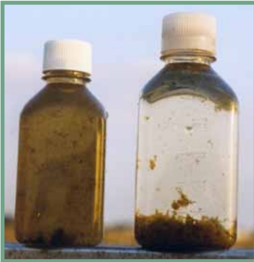
Figure 8: Demonstration of the effect of coagulant and flocculant on Maribrin Farm effluent. (photo STM aquatrade)
