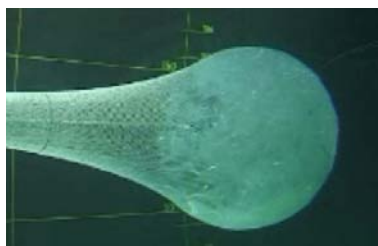
Figure 1.3: View of a cod-end in a flume tank; the fish is replaced by plastic bags filled with water
