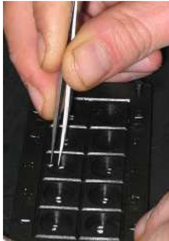
Figure 20 : Placing the otoliths from small pelagic fish in the cavities of a black plastic strip.
