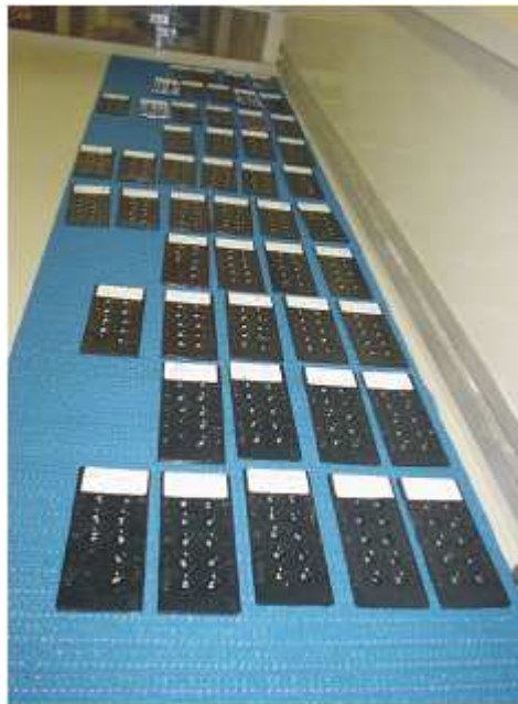
Figure 21 : Strip with the cavities containing sardine otoliths and filled with Eukitt resin.
