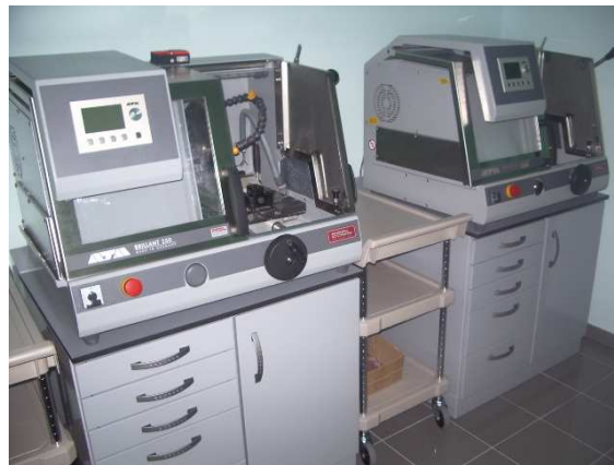
Figure 28 : Automatic high speed Escil Brillant 250 ® .
