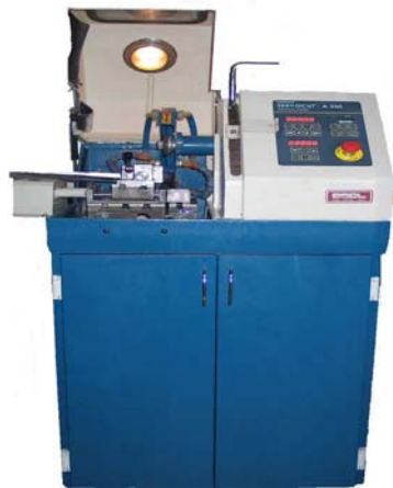
Figure 27 : Automatic high speed ESCIL Servocut A250 ® saw.
