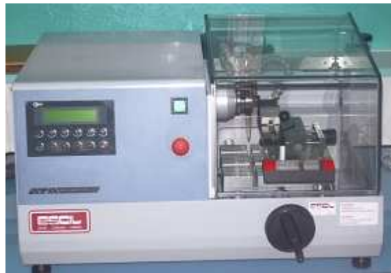
Figure 30 : Escil automatic variable speed Brillant 221 ® saw (400 to 6000 rpm).
