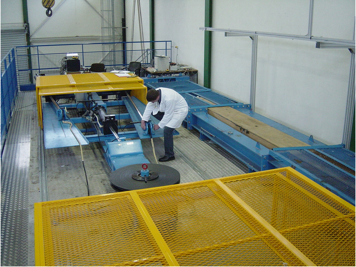
Fig. 3. Cable test facility. Foreground bend-over-sheave machine to test high performance ropes on oceanographic sheaves, background 100 ton capacity cable tensile test frame.
