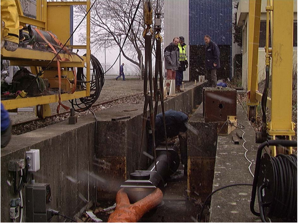
Fig. 2. Central interface element connecting steel and polyester ropes during torsion interaction tests.
