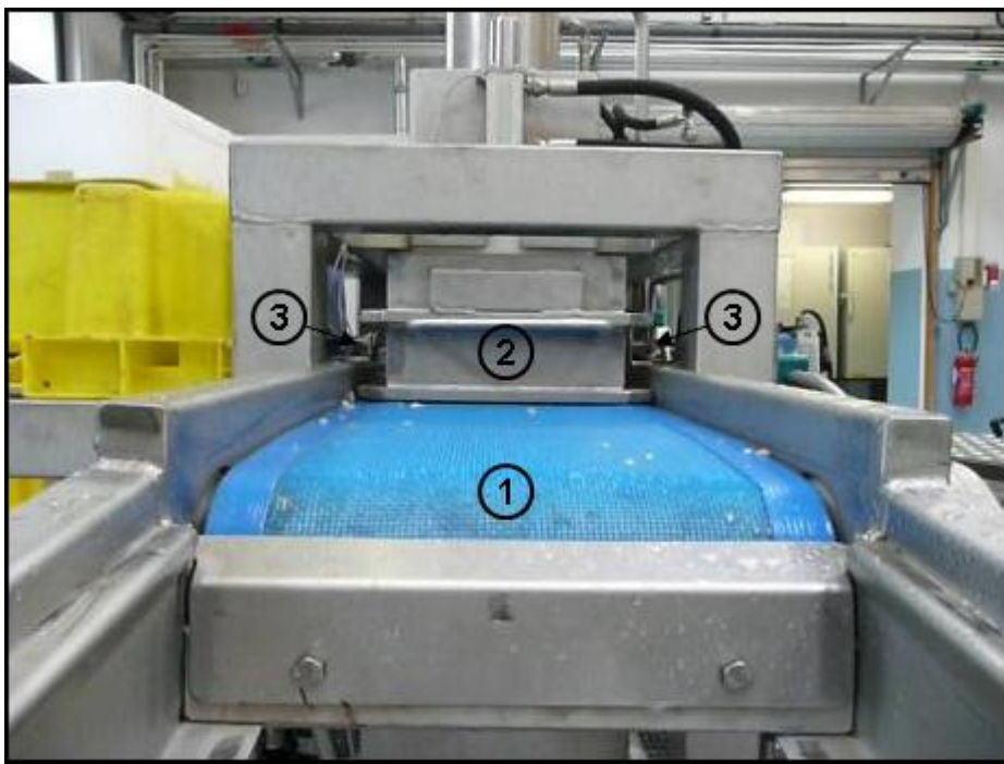
Figure 3.6. View of the belt conveyor (1), steel mould (2) and motion detectors (3).
