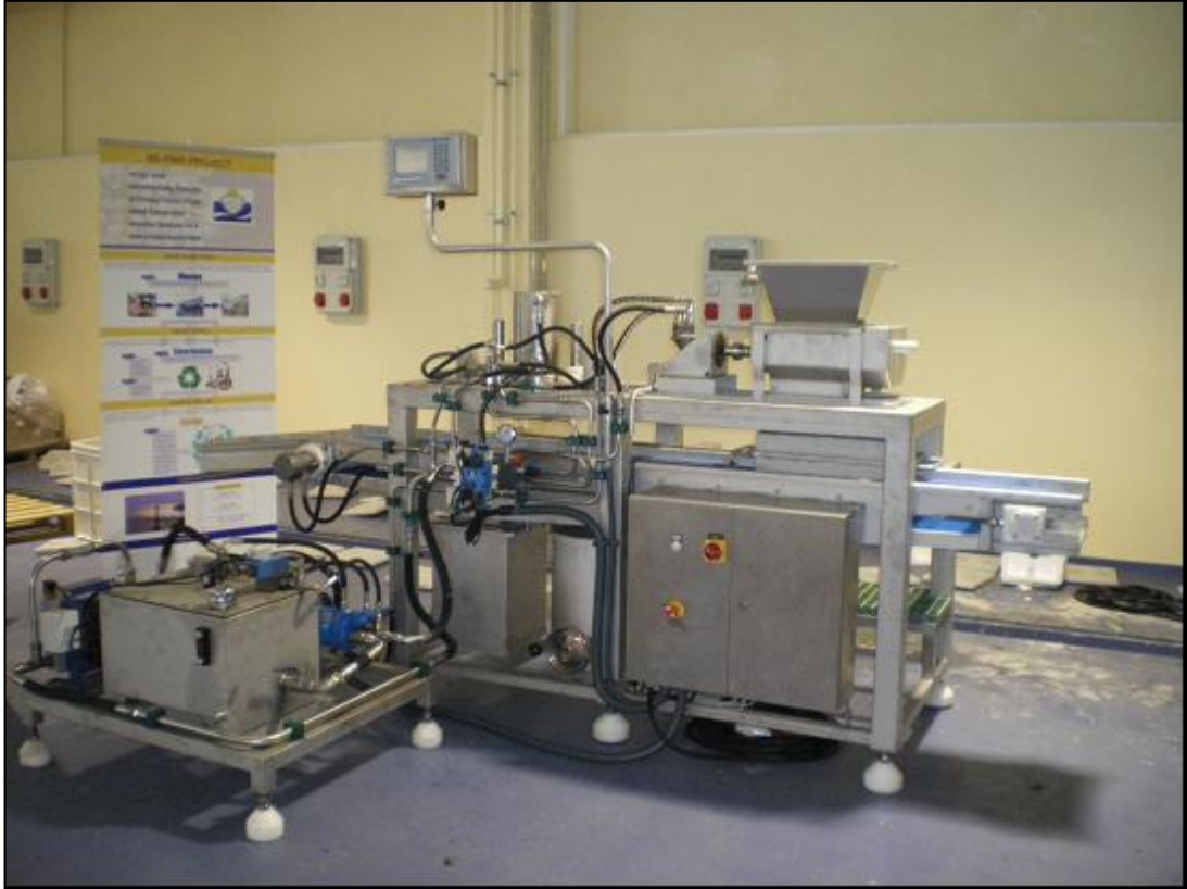
Figure 3.3. Frontal view of the prototype and the hydraulic power station.
