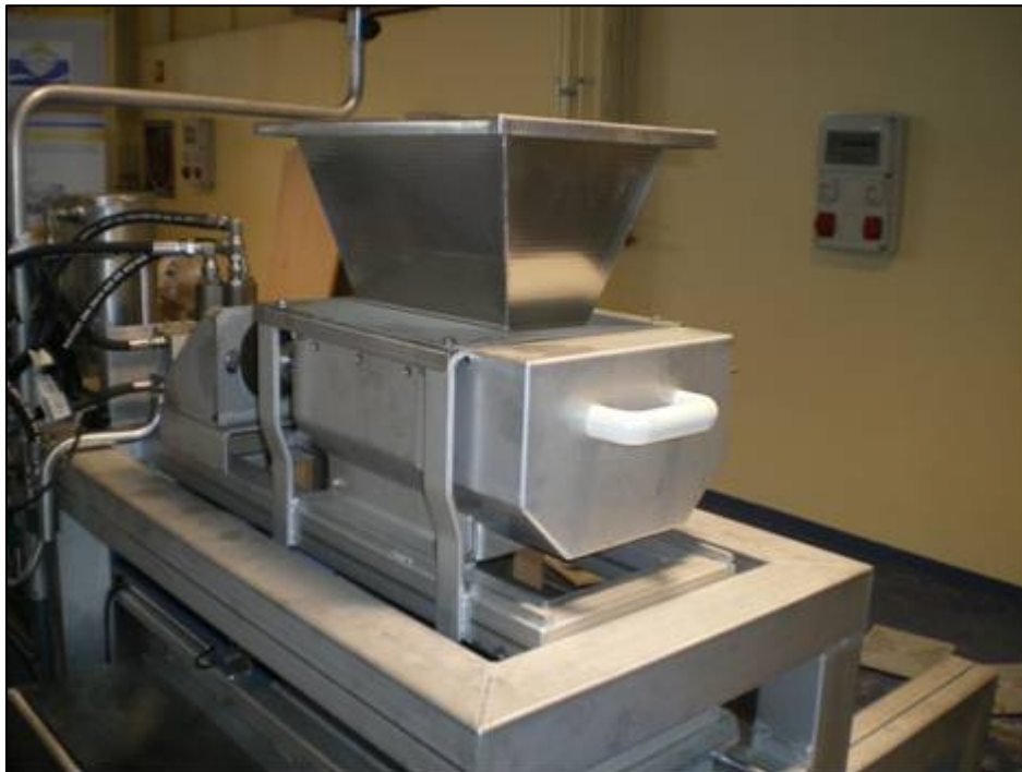
Figure 3.5. Frontal view of the prototype and the hydraulic power station.
